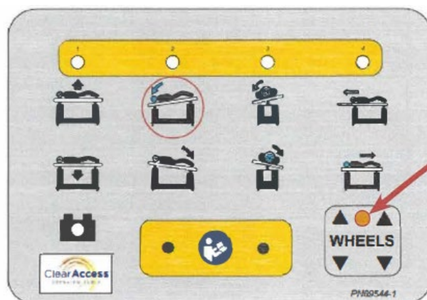
Figure 9: The WHEELS light on the Fixed Control Panel at the Foot-End of the Table
