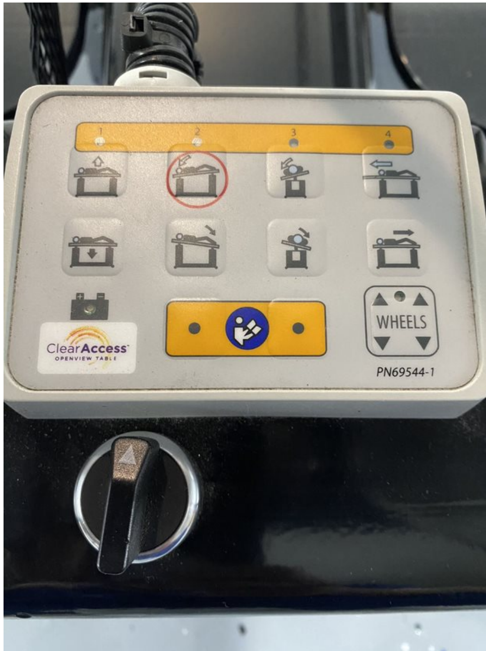
Figure 8: ON/OFF Switch enables/disables all controls to the Table. The ON/OFF Switch is shown in the ON position (controls enabled).
